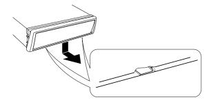
The frame can be removed from the bottom side in the same manner.
